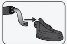
1. Line up holes to desired position and insert boat roller bar into suction cup. Bar can be mounted upright or at a 90° angle.
