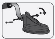
2. Insert bolt through aligned holes, Install nut and tighten.
